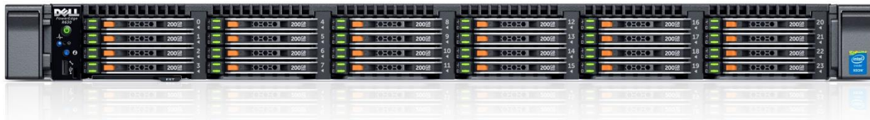
Figure 3. 24-drive bay chassis front view without bezel
