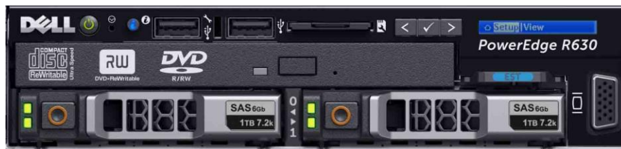
Figure 7. LCD control panel for 8-drive bay chassis
