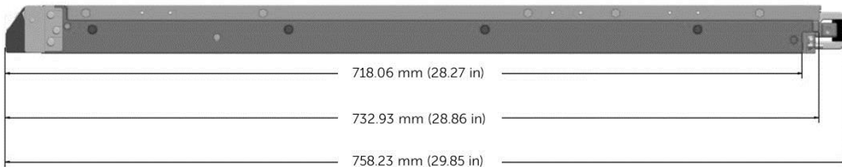
Figure 24. Chassis depth without bezel for 8-drive chassis option
