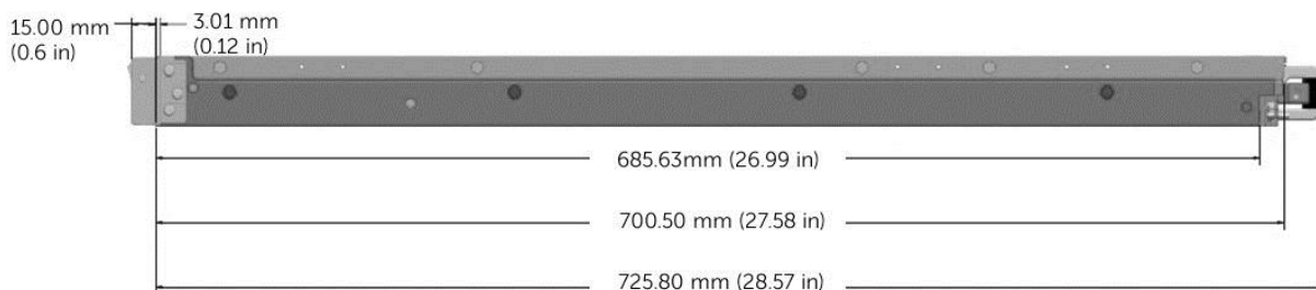
Figure 24. Chassis depth without bezel for 8-drive chassis option
