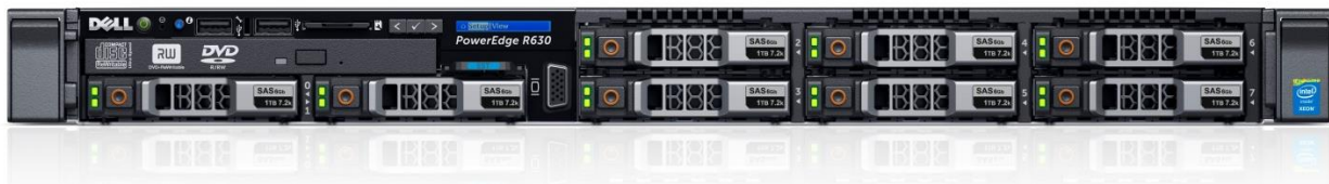
Figure 1. 8-drive bay chassis front view without bezel
