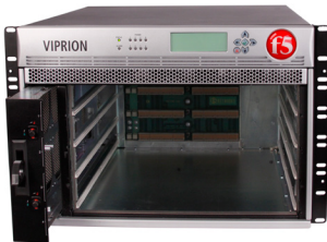
VIPRION 4480 Chassis (fan tray)
