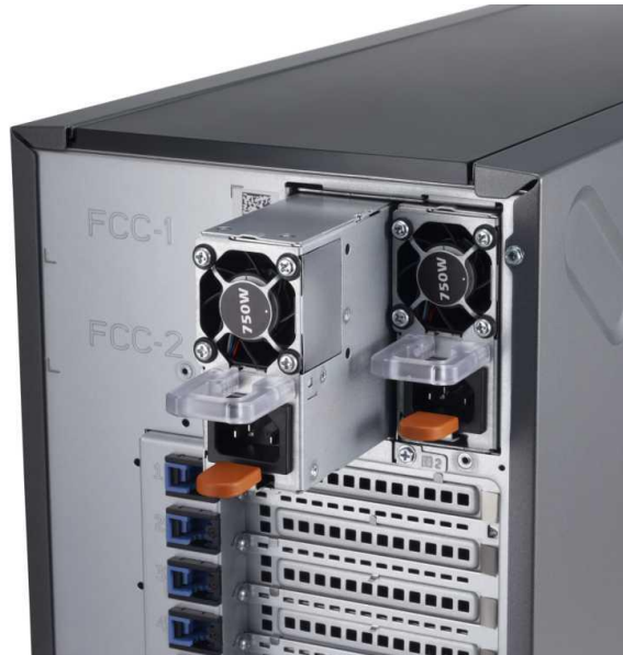
Figure 8. 750W power supply unit
