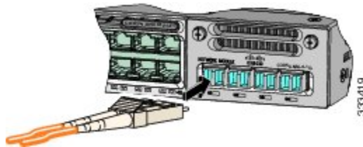
Figure 8: Network Module with SFP Modules Installed
