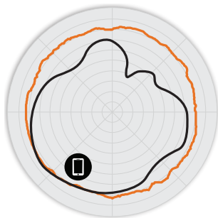
Figure 2. M510 2.4GHz Azimuth Antenna Patterns
