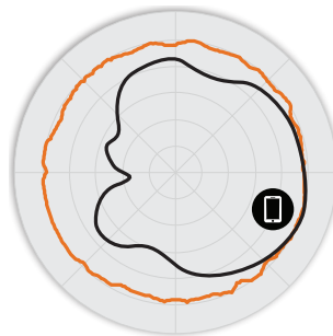
Figure 3. M510 5GHz Azimuth Antenna Patterns
