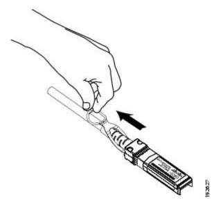
Step 2 Insert the optical SFP+ transceiver into the FEX port. Make sure that it clicks firmly into place.
