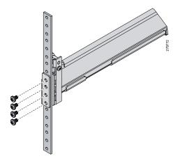
**Step 5** Follow the same procedure to install the other rack rail as shown below.
