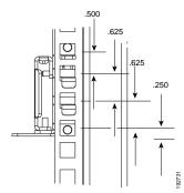
The following figure shows a rail mounted into a rack in the proper position with respect to a rack-unit boundary. Measurements are in inches between the centers of the holes.
