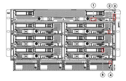
Figure 15: LEDs on a Cisco UCS 5108 Server Chassis—Front View
