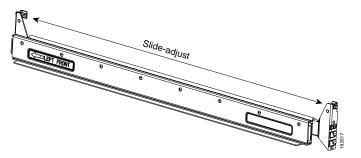
Step 3 Place the two hooks at each end of the rail into the first two holes at a rack unit boundary.
