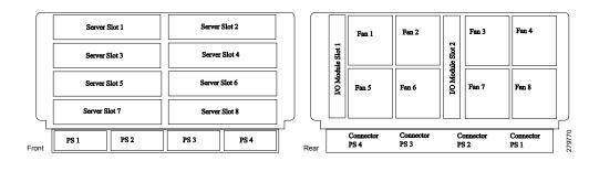
Figure 41: Power Supply Bay and Connector Numbering (AC Version Shown)
