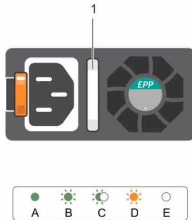
Figure 8. AC power supply status indicator
