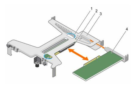
Figure 35. Removing and installing the expansion card from the expansion card riser
