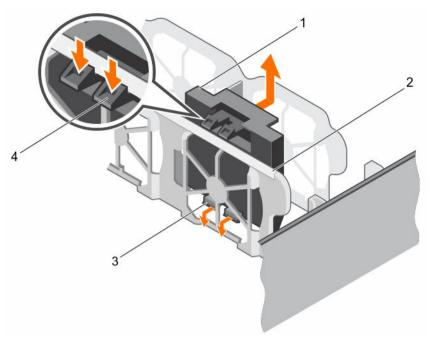
Figure 31. Removing and installing a cooling fan blank
