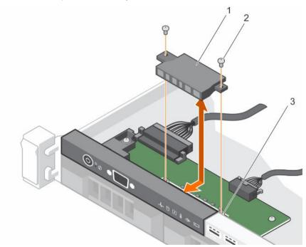
Figure 50. Removing and installing the LED module—four cabled hard drive chassis
