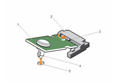
Figure 54. Installing the TPM
