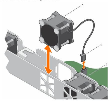
Figure 32. Removing and installing a cooling fan
