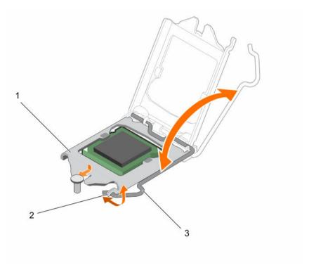
Figure 40. Opening and closing the processor shield
