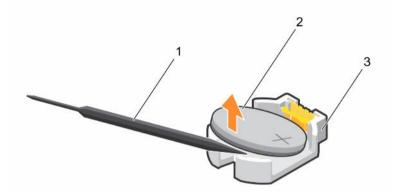
Figure 44. Removing the system battery
