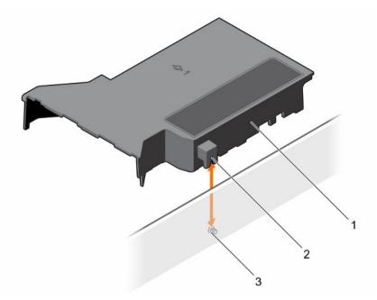
Figure 15. Removing and installing the cooling shroud
