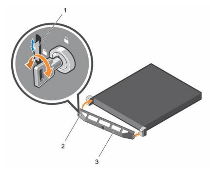
Figure 9. Removing and installing the optional front bezel
