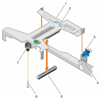
Figure 34. Removing and installing the expansion card riser
