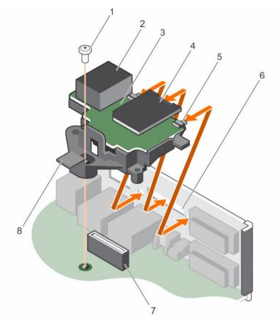
Figure 38. Removing and installing the iDRAC port card
