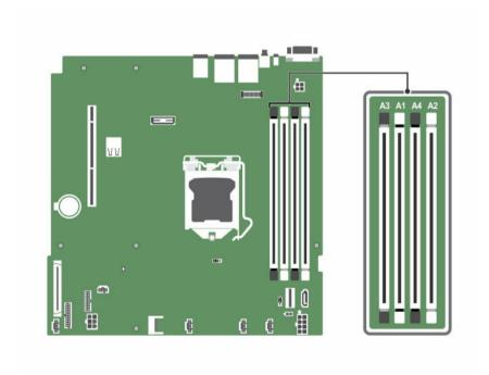
Figure 16. Memory socket locations on the system board
