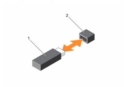
Figure 33. Replacing the internal USB key
