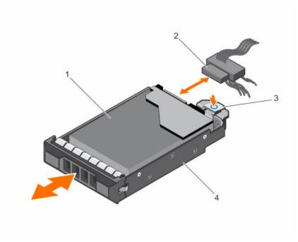
Figure 20. Removing and installing a cabled hard drive carrier
