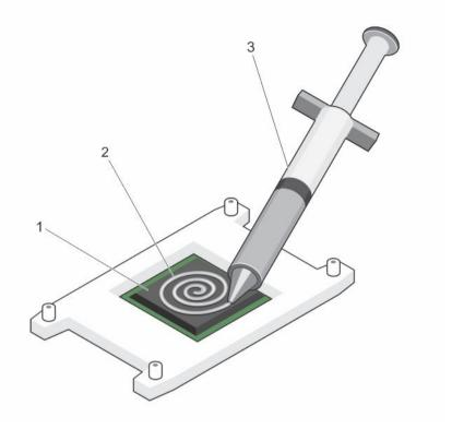
Figure 42. Applying thermal grease on the top of the processor
