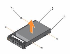
Figure 23. Removing and installing a hot swappable hard drive into a hard drive carrier
