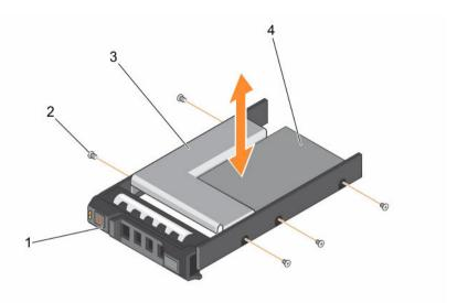
Figure 25. Removing and installing a 3.5-inch hard drive adapter into a 3.5-inch hot swappable hard drive carrier
