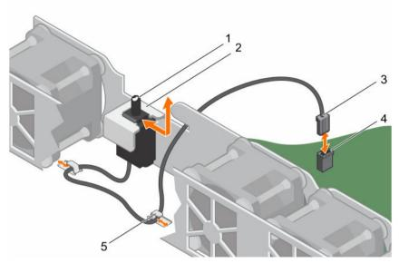
Figure 14. Removing and installing the intrusion switch
