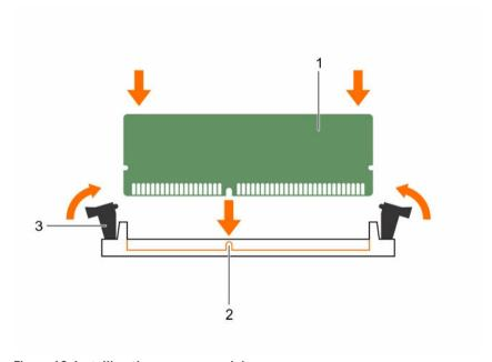
Figure 18. Installing the memory module
