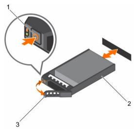
Figure 22. Removing and installing a hot swappable hard drive carrier
