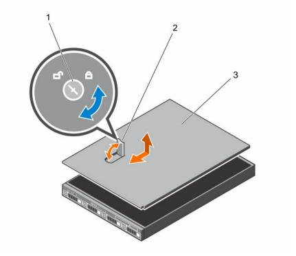
Figure 10. Removing and installing the system cover
