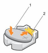
Figure 45. Installing the system battery
