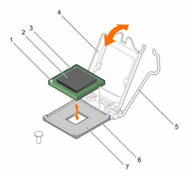
Figure 41. Removing and installing a processor
