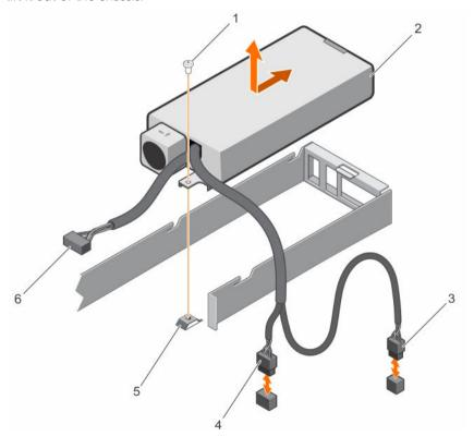
Figure 43. Removing and installing a cabled power supply unit
