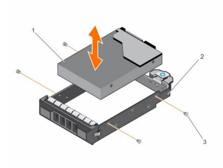
Figure 21. Removing a cabled hard drive from a cabled hard drive carrier
