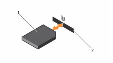
Figure 37. Removing and installing the SD vFlash card
