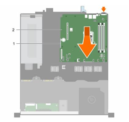
Figure 53. Removing and installing the system board
