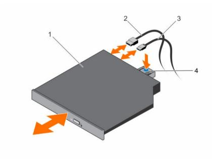
Figure 30. Removing and installing the optical drive
