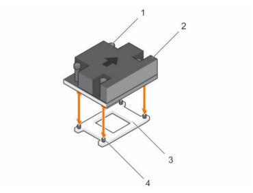
Figure 39. Removing and installing a heat sink
