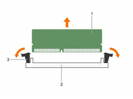
Figure 17. Removing memory module
