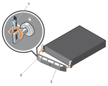
Figure 9. Removing and installing the front bezel
