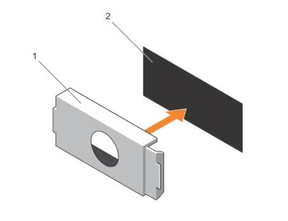
Figure 37. Removing and installing the power supply blank
