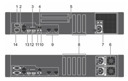
Figure 4. Back-panel features and indicators for a non-redundant power supply unit chassis and a redundant power supply unit chassis
