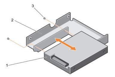
Figure 20. Removing and installing a 2.5 inch hard drive into a 3.5 inch hard-drive adapter
