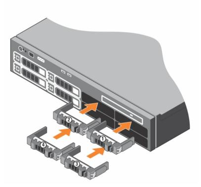
Figure 19. Hard-drive blank installation sequence
