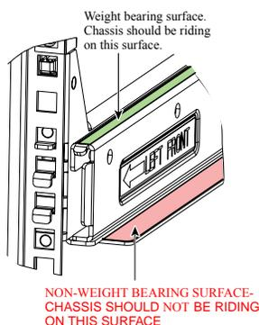
**Caution** The mounting rails may come loose and cause the chassis to fall if the weight is resting on the wrong surface. Make sure that the bottom of the chassis is resting on the correct rail surface.
