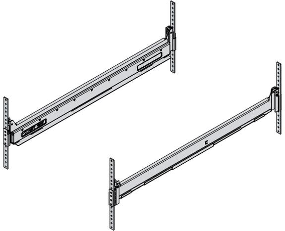
**Step 6** Use a tape measure and level to verify that both rack rails are horizontal and at the same height.
