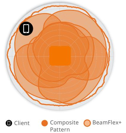
Figure 2. T310d 2.4GHz Azimuth Antenna Patterns
