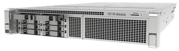
Cisco 8540 wireless LAN controller supports several buttons, LED indicators, and a KVM connector on the front panel. It includes a power button and Locator LED button, along with the following LEDS: System status, PSU status, Fan status, Network LED, and Temperature LED.
