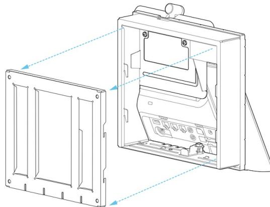
The following diagram illustrates how to attach a Cisco IP Phone 8800 series with a key expansion module to your wall bracket.
