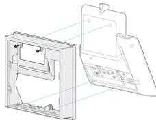
The following diagram illustrates how to attach a phone bracket to a Cisco IP Phone 8800 series phone equipped with a key expansion module.
