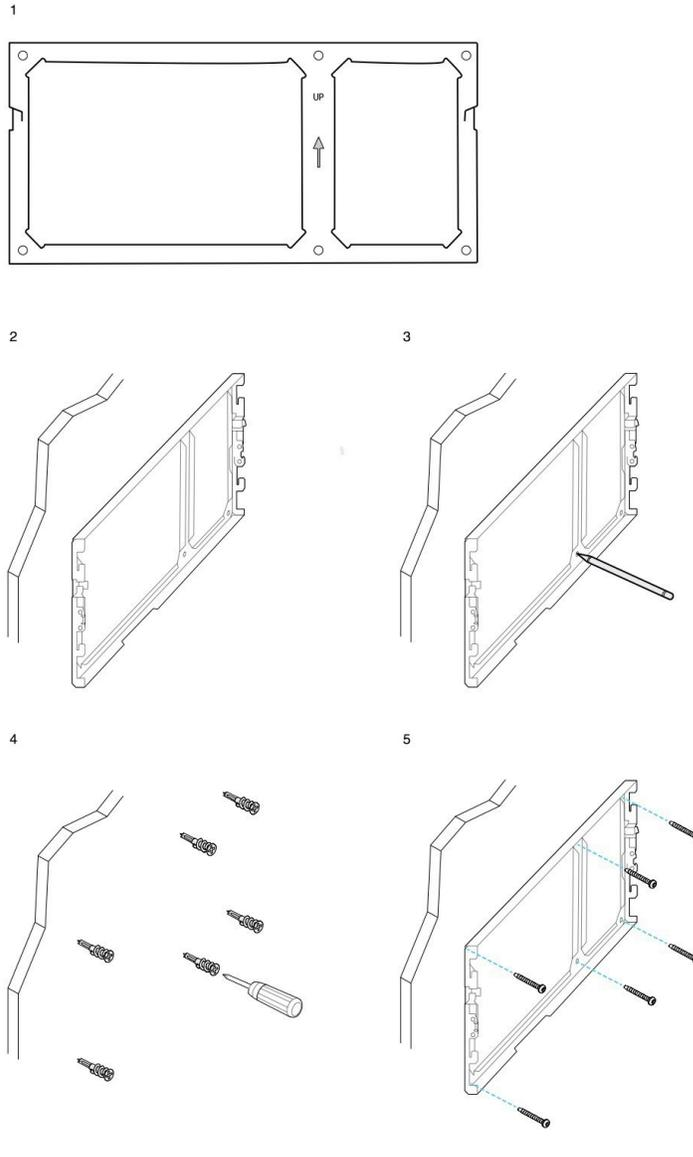
The following diagram illustrates step 2 to step 5 of attaching a Cisco IP Phone 8845 and 8865 series wall bracket to a wall.
