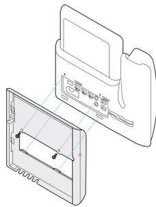
The following diagram illustrates how to attach a Cisco IP Phone 8845 and 8865 to a phone bracket.
