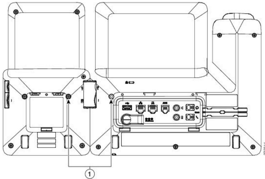
**Note** Make sure that the screws are fully inserted into the phone and tightened.
