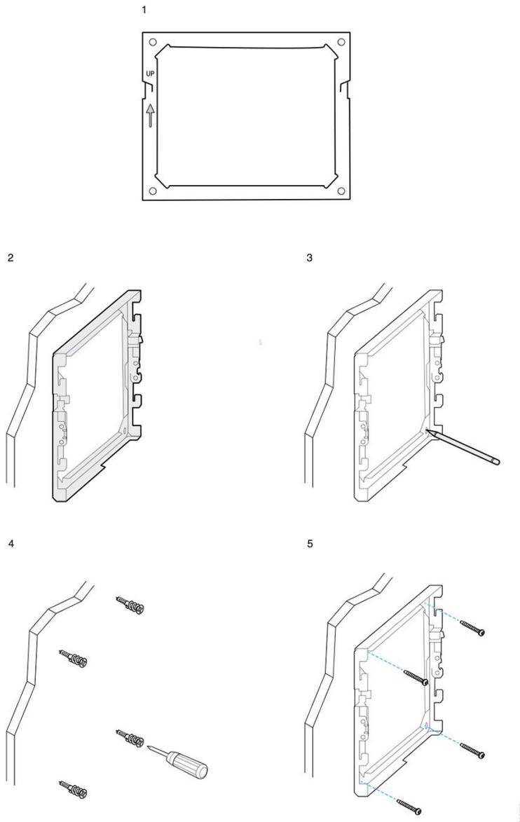
The following diagram illustrates attaching a Cisco IP Phone 8800 series wall bracket with a key expansion module to a wall.
