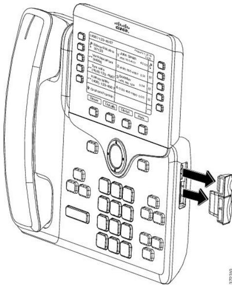
**Caution** The slots are designed for the spine connector only. Insertion of other objects will cause permanent damage to the phone.
